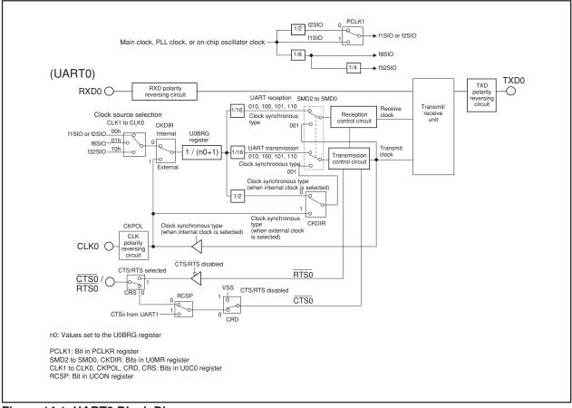
Figure 14.1 UART0 Block Diagram
